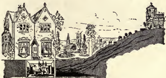
Fig. 636. Vicarage rendered unhealthy by infiltration from church-yard.
